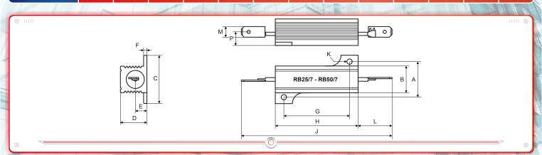
Fixed power wirewound resistors aluminium housed with screw leads (TOP)
